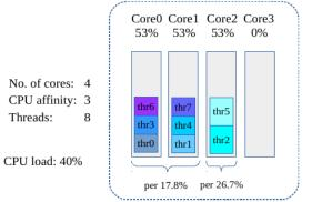
Figure 3: Unison thread and load distribution onto the cores
