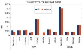
Figure 2: Opcode mix of VLC player vs. vidplay load model.
