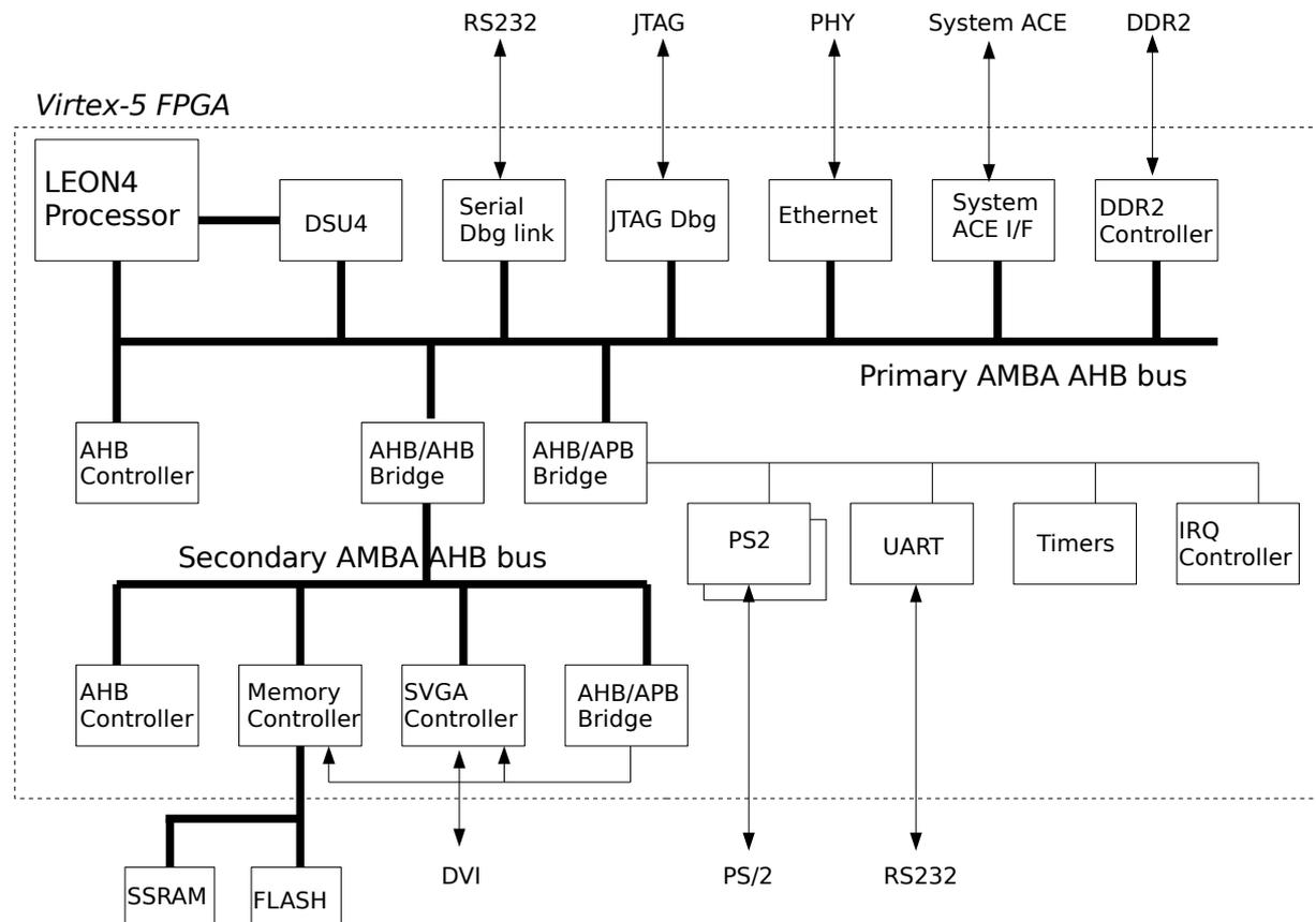
Figure 1: Block diagram of a LEON4 SoC for FPGA prototyping
