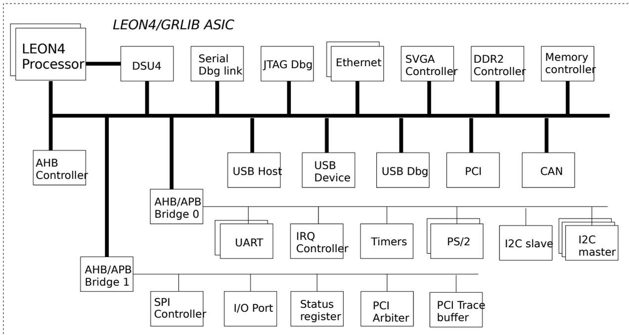
*Figure 2: Block diagram of the LEON4 based evaluation SoC ASIC*
