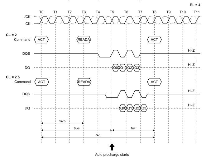
Figure 8-2. Read Cycle with Auto Precharge
