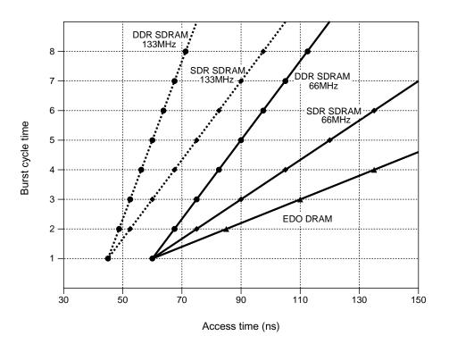
Figure 3-7. Access Time of DDR SDRAM, SDR SDRAM and EDO DRAM
