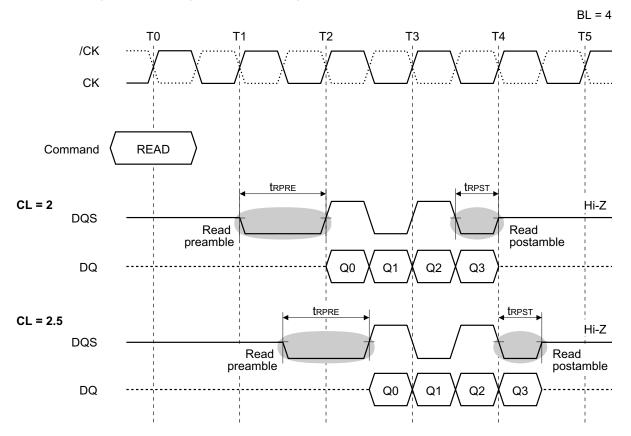
Figure 9-6. Timing of Data Strobe Signal Read Preamble and Read Postamble 1
