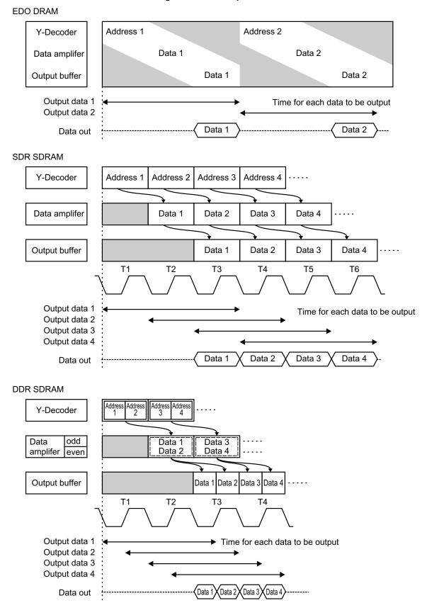
Figure 3-5. Burst Operation
