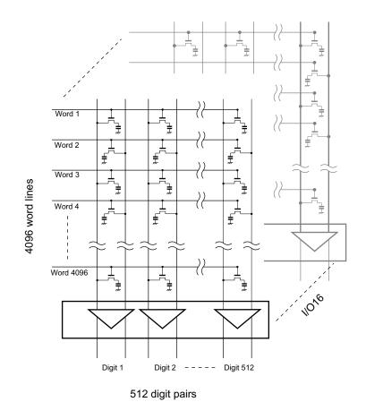
Figure 2-4. Memory Cell Array of 128M bit DDR SDRAM (EDD1216ALTA) (Bank A)
