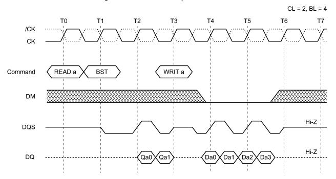
Figure 12-4. Read/Burst Stop/Write Command
