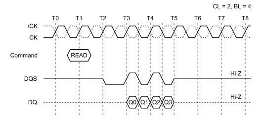
Figure 1-4. DDR SDRAM Read Cycle Timing
