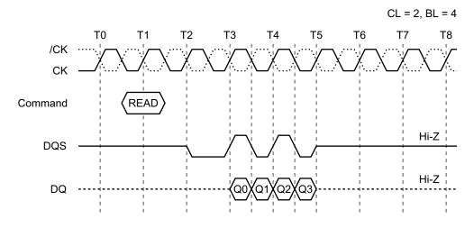
Figure 3-1. DDR SDRAM Read Cycle Timing
