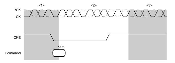
Figure 11-2. Example of Clock Enable Signal Control
