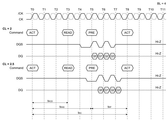
Figure 8-1 shows the basic operation timing chart for the read cycle when the burst length = 4.
