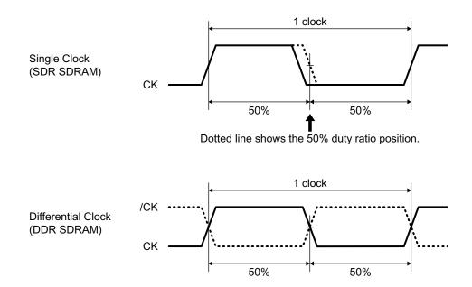
/CK is an input signal that has the same clock period but the reverse phase of CK. The high-level period and lowlevel period can be made equal by using the intersection of CK and /CK as an input reference level. In the case of DDR SDRAM, data input/output is synchronized with both the rising and falling edges of the data strobe signal (DQS), which has the same period as clock input CK.
