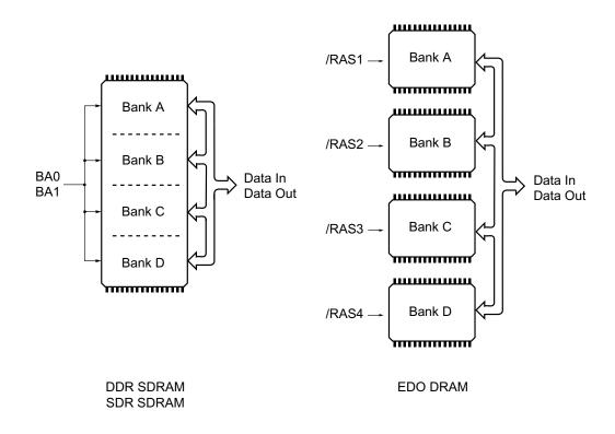
Figure 3-4. Four-Bank Configuration
