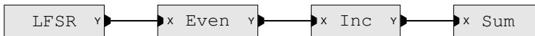
Fig. 10. A program with four processes. LFSR is a linear feedback shift register, producing the n = 10^7 first numbers of a maximum length sequence of 16 bits, followed by a 0. Even filters out all odd values, forwarding only the even numbers to Inc , that increments the numbers by 1. Sum computes the sum of all numbers until it gets a 1 (the incremented 0 at the end of the stream) and prints the sum.
